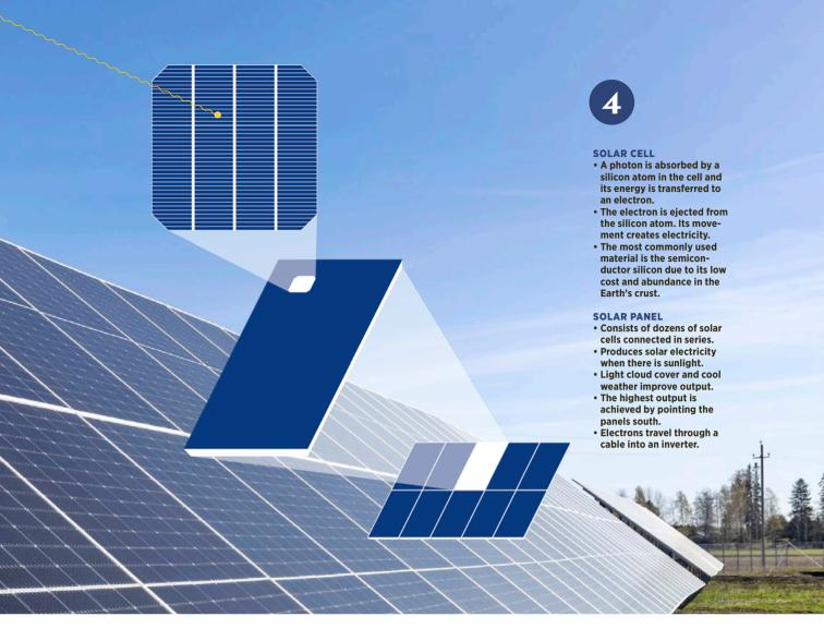
usually blue and their structure is visible in the form of crystals of different sizes on the surface of the cell. Monocrystalline panels are darker, or completely black. Their conversion efficiency is currently the highest at 21-22%.
